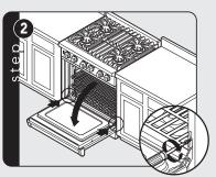
Open door completely. Reinstall hinge trim.
